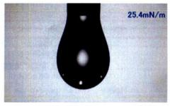
Inversion measurement with inverted needle is possible. It is usable in the case that liquid of low density is scarce or colored in interfacial tension measurement, a measurement by discharging air bubble in liquid is preferable.
