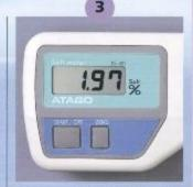
After arrow flashes three times, the display indicates the salinity of the measured sample in percentage.
