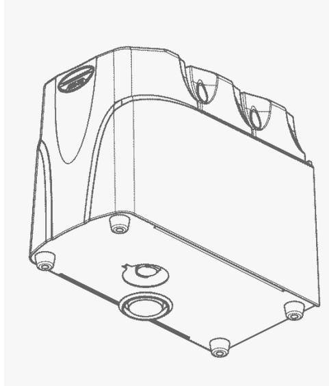
Open the battery cover on the bottom of the main unit with a slotted screwdriver. Replace the old battery with a new one (CR2032).
