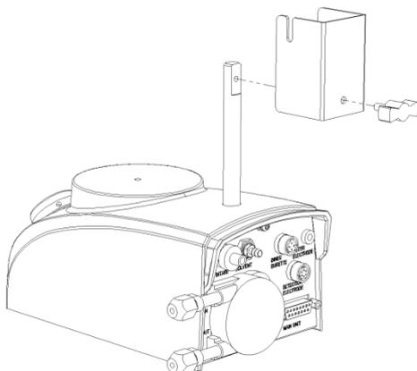
4) Fix the titration cell to the cell holder.
