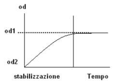
A single reading that reaches a constant optic density at the end of the reaction.
