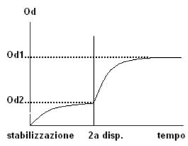
A single reading that reaches a constant optic density at the end of the reaction. Each reaction is based on two dispensations. As for our enzymatic determinations, the configuration commonly determines R1+sample in a first dispensation and R2 in a second.
