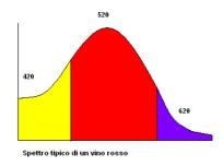
To the side is the typical spectrum of a red wine at the three wavelengths. As the printed result shows the absorbencies of each single wavelength, it is possible to determine the percentage contribution of each single wavelength out of the total:
